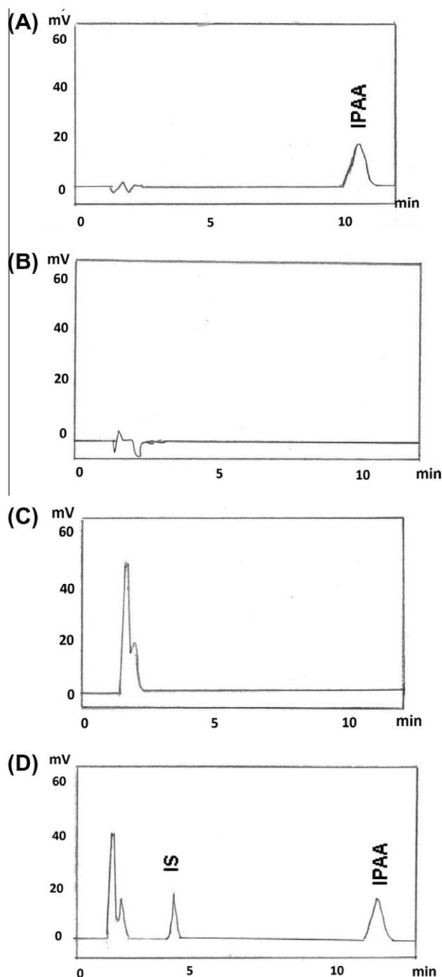
**Fig. 1.** Tracings in HPLC chromatograms of formulations and standard. (A) Vitamin derivative, ascorbyl tetra-isopalmitate (IPAA). (B) Reagent control (isopropanol). (C) Formulation IPAA-free. (D) Formulation containing IPAA and the internal standard vitamin K1 (IS).
